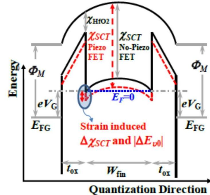
The gate controlled strain in the semiconductor implies a gate controlled electron affinity that results in the simplified SS expression
