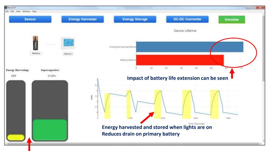
Dynamic visual aid to see charge and discharge on supercap when lights are on/off
