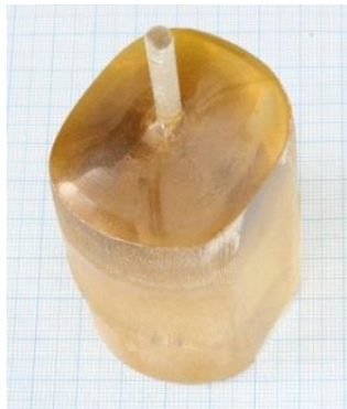
Semi-insulating Mg-doped Ga 2 O 3 crystal (2")
