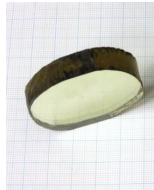
Ga 2 O 3 slab, 1 cm thick cut out from boule
